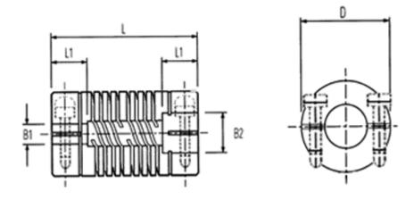
B2: Pre-drilled = 8.0B2: Pre-drilled = 10.00= M4Cap screw D = 31.8 L = 57.2 L1 = 16.0Max angular displacement = 0.50 = 16.00
